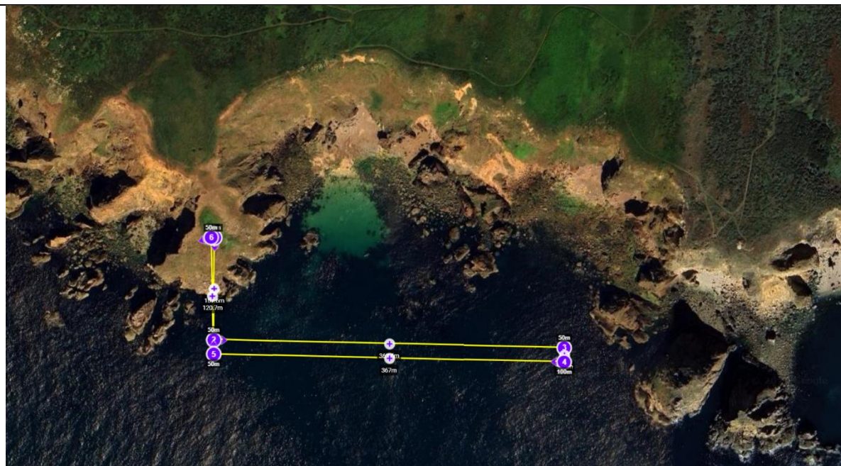
Figure 1. Example of potential flight path for pilot drone survey of nesting seabirds on Alderney’s South cliffs. The pre-programmed path runs parallel to the coastline, flying at multiple altitudes to achieve 60% vertical overlap and ensuring birds obscured by overhanging rocks, vegetation or rock formations are visible. The flight pattern will be pre-programmed with autonomous flight planning software, e.g. ‘Litchi’.
