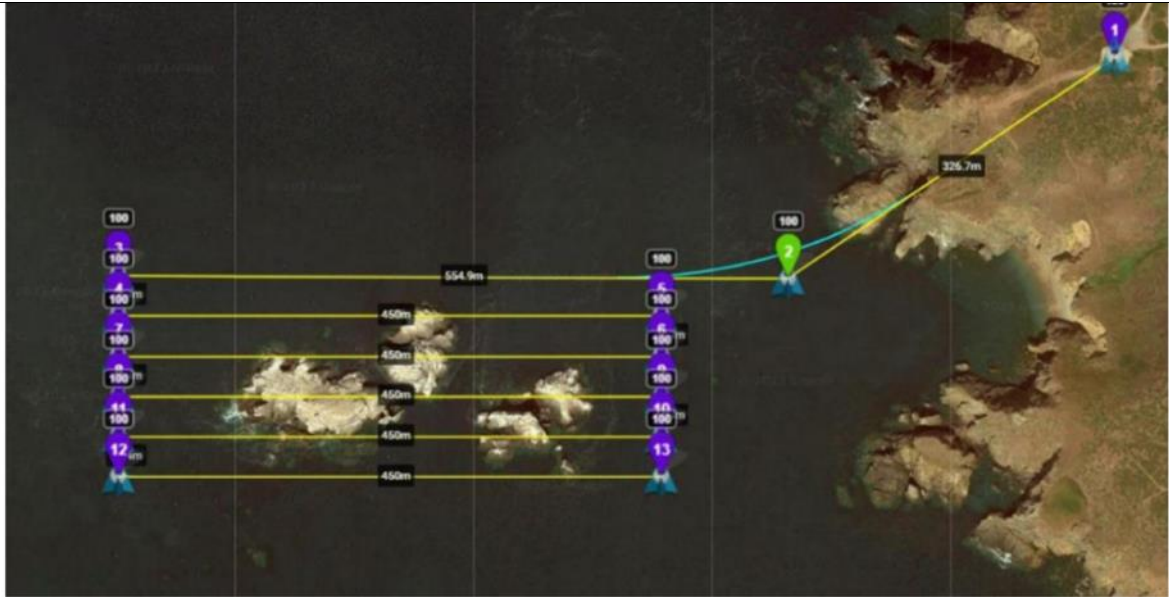
Figure 2. Example of potential flight paths for drone survey of Les Etacs following a lawnmower (grid) flight pattern, with 60% sideways overlap to ensure that no part of the colony is missed. The flight pattern will be pre-programmed with autonomous flight planning software, e.g. ‘Litchi’. The pilot will be able to use the cameras viewfinder, and take direct control of the drone, to view suspected rodents.
