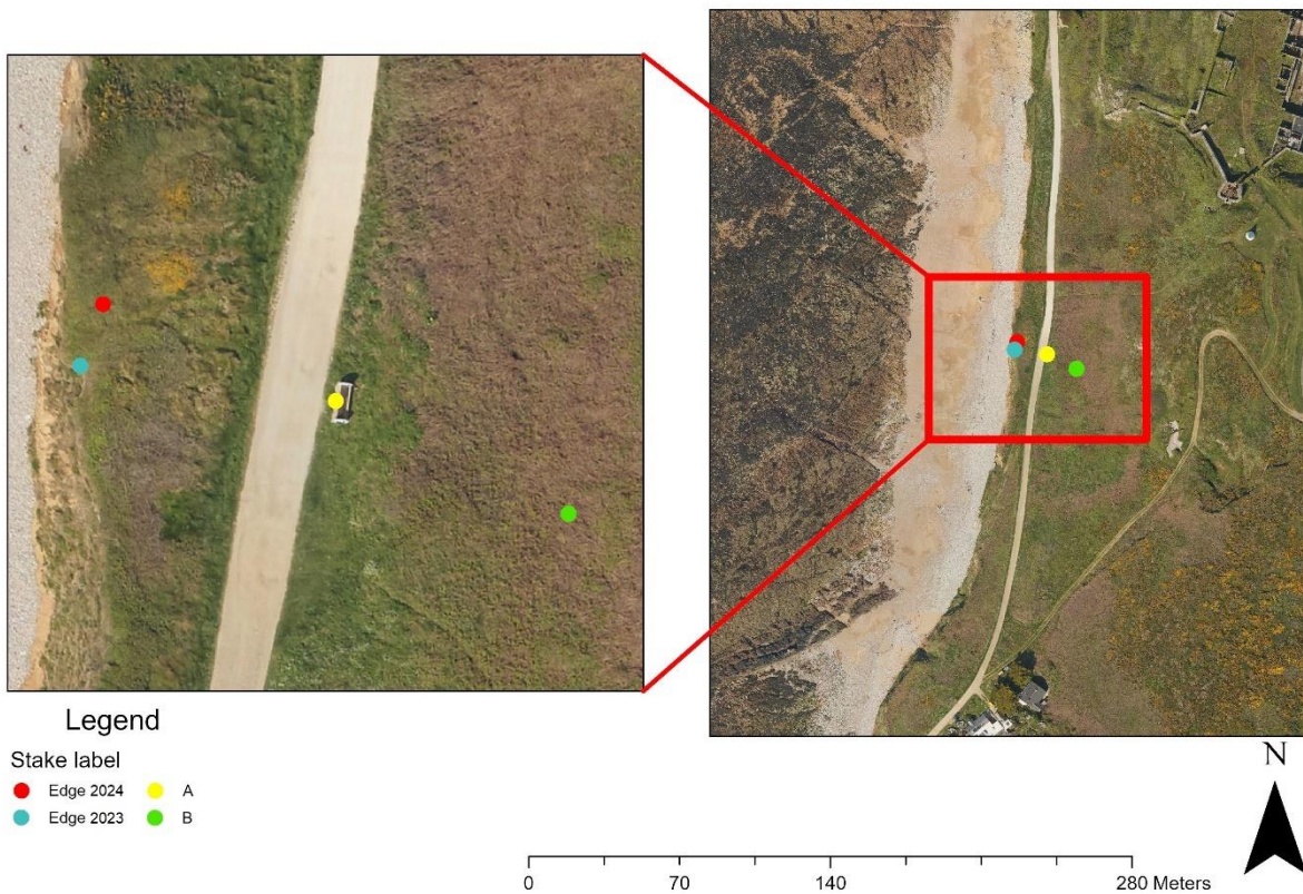
Figure 15. Location of the monitoring station transect and individual stations (edge, A and B stakes/stations) with observed coastal erosion at Clonque Bay. Edge monitoring station in 2023 was lost, with a new edge station added in 2024. Aerial photograph provided by Digimap Ltd. Coordinate system: Guernsey Grid.
