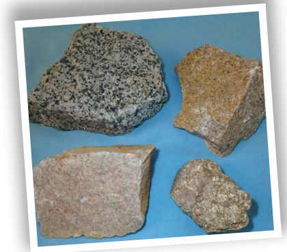
FIG. 2. CLOCKWISE FROM TOP LEFT, GRANODIORITE, TELEGRAPH BAY GRANITE, MICROGRANITE AND APLITE. | JUSTIN HART
