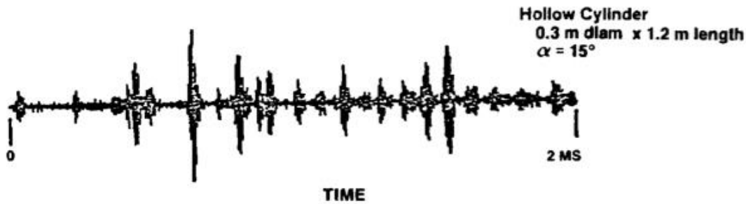
Figure 4: Received echoes of Bottlenose dolphin from a hollow cylinder (Au W. S., 1980).
