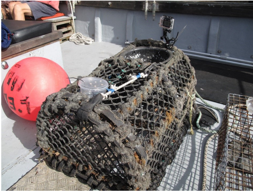
BRUV 2: Lobster pot with attached camera and bait box (photo credit S Robertson)
