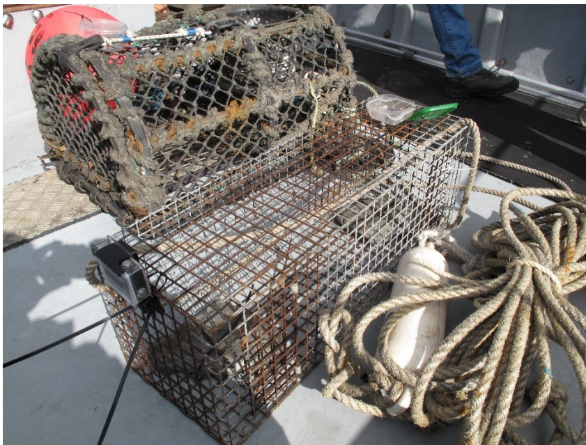
BRUV 1: Cage with attached camera and bait box (photo credit S Robertson)
